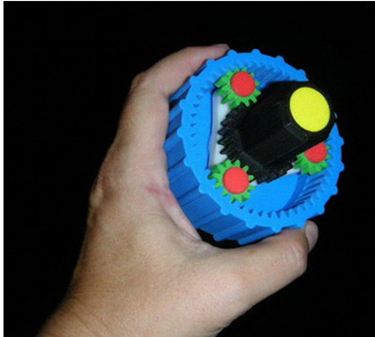
Figure 5-12 - Fused deposition modeling, colored ABS functional model (Source: Stratasys)
