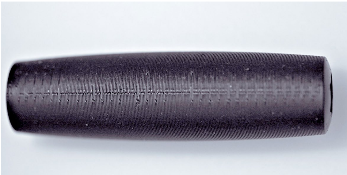
Figure 5-8 - Joint line on extrusion processing. (Source: CP-GmbH/FH-Aachen)
